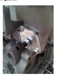
4. Slowly start turning in the adjustment screw. You will see the slack starting to go away. As the chain gets tighter, use a ruler to measure the slack. Push the chain down and pull it up will little force. Tighten the tensioner so there is roughly 1/4" of slack.
