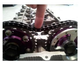
3. With the piston bottomed out inside the tensioner, install the assembly. Make sure the slot in the piston lines up with adjustable timing chain guide. You will have to look down the timing chain valley to verify. Improper alignment will cause engine damage. Also, we suggest installing a new gasket.
