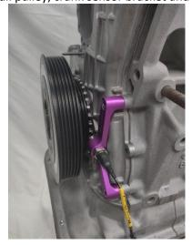
6. Install block off where the FWD distributor used to go.
