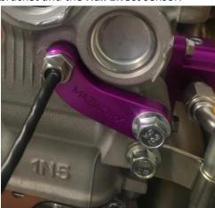
2. Install the Cam Angle Sensor Wheel on exhaust cam. You will have to change the dowel pin on the cam to the longer one. Use longer bolt supplied to mount wheel and cam gear to cam.
