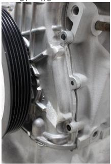
5. Install pulley, crank sensor bracket and the Magnetic Sensor.
