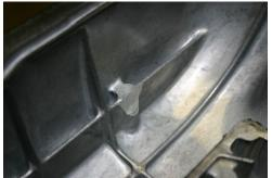
4. Before installing pulley, grind the ribs on the front cover to clear the bracket and sensor.
