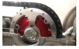
3. Grind inside of the valve cover to clear Cam Angle Sensor Wheel as shown. Verify clearance.
