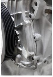
2. Install pulley, crank sensor bracket and the Magnetic Sensor.
